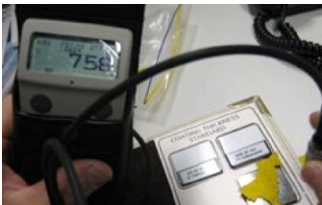
Dry film build testing of over applied Roadmarking coating. Still soft after 3 weeks of application and not curing.
