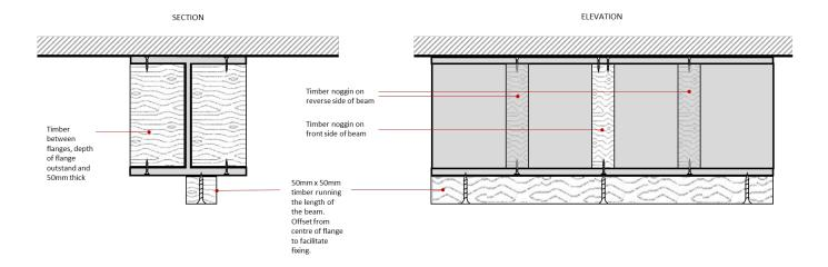
This arrangement was tested to evaluate encasement attached via 2 inch (50mm) width timber/wooden noggins or batons, and other attachments to the fire protected beam using a similar attachment method.
