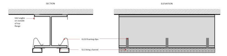
The attached items caused no significant detriment to the fire protection of the beam.
