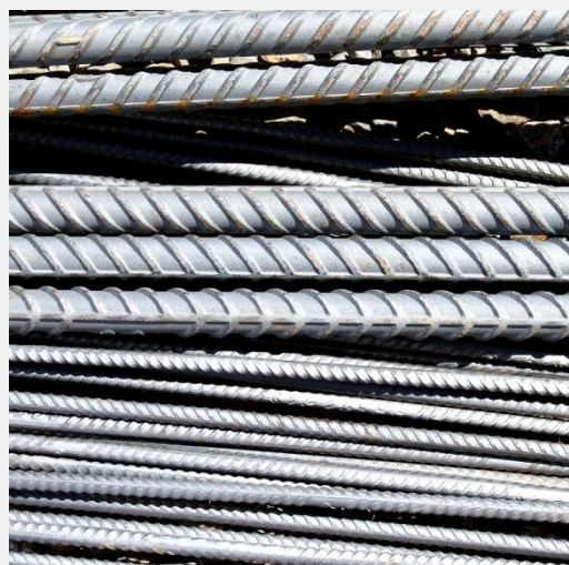
Steel and concrete expand and contract at the same rate – perfect partners!
