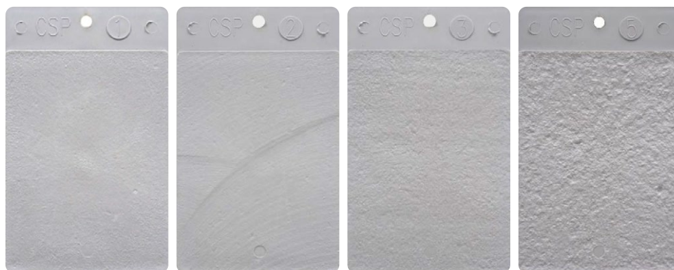
Figure 1: Concrete Standard Profiles from left to right. CSP 1, CSP 2, CSP 3, and CSP 5.
