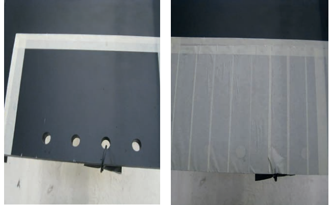
Folded masking tape on perimeter area/folded masking tape area with normal masking infill, (single coat application).
