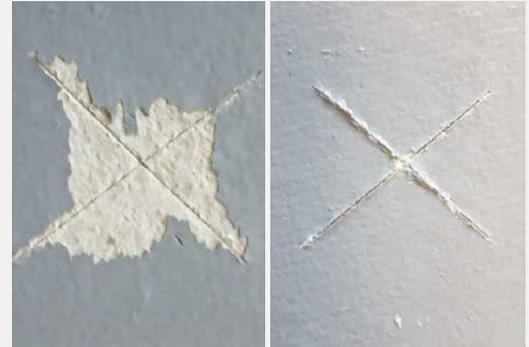
*Adhesion tests clearly show strength of adhesion of the existing coating to the substrate. If there is any doubt, complete removal is the best option.*
