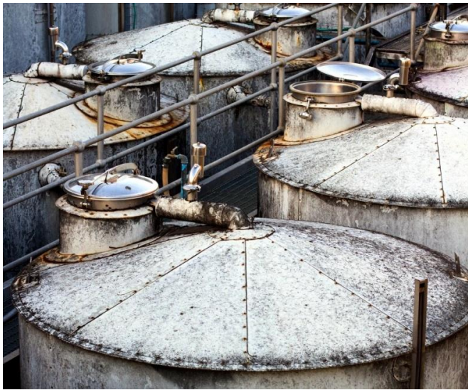
The cladding's zinc layer has corroded to white zinc oxide. Red rust shows where the zinc has been completely depleted.
