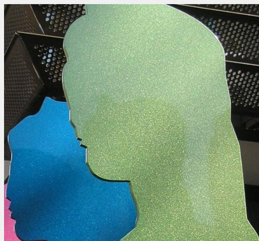
*Quantum FX metallic polyurethane shows a highlevel of metallic flip*
