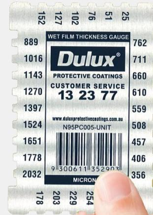
*The Dulux Protective Coatings wet film gauge or wet film comb*
