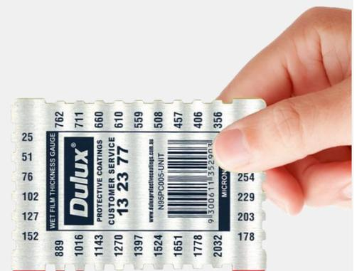
*The comb has red paint on the first two teeth, 889 and 1016 µm but none on the 1143 µm tooth, showing that the coating is at least 1016 µm*
