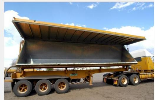
Large, heavy rocks are dropped into these Kiernan Transport tippers without damage, saving maintenance costs
