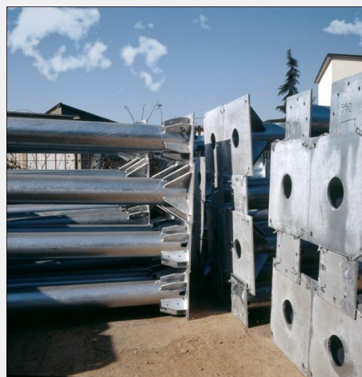
The sacrificial process starts immediately on exposure – white rust is visible on unprotected areas
