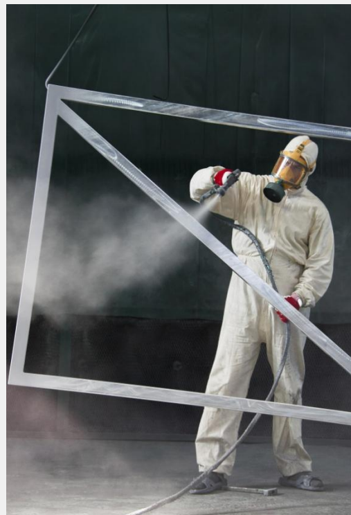
Solvent vapours are avoided by use of air fed face respirators. Over-spray accounts for most wastage in the spray painting process
