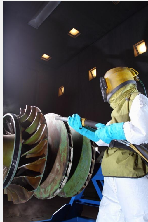
Abrasive blast cleaning can be used on new or old steelwork, and is very fast and efficient. Sand blasting is no longer permitted
