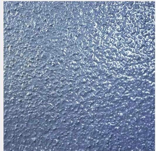
*The coarser a floor, the greater the slip resistance, but only if the floor can be kept clean and free of greasy deposits.*
