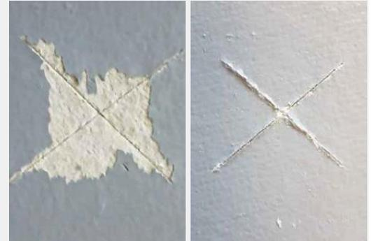
*Adhesion tests clearly show strength of adhesion of the existing coating to the substrate. If there is any doubt, complete removal is the best option.*
