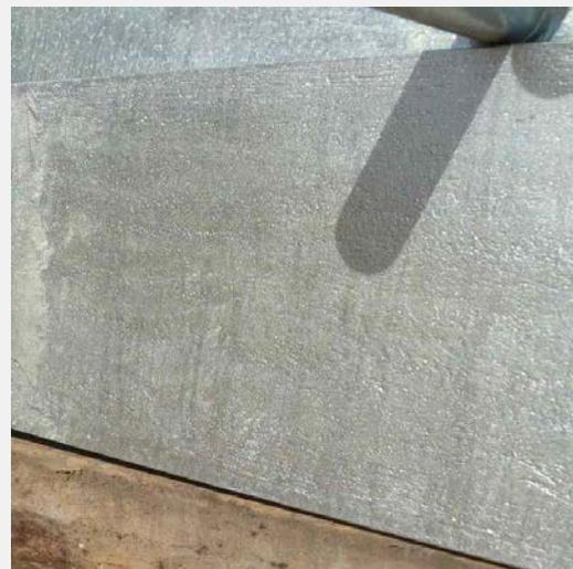
*The more uniformly dull the surface, the better for coating adhesion. Coatings must be applied immediately after cleaning to minimise surface recontamination from atmospheric salts and zinc corrosion*
