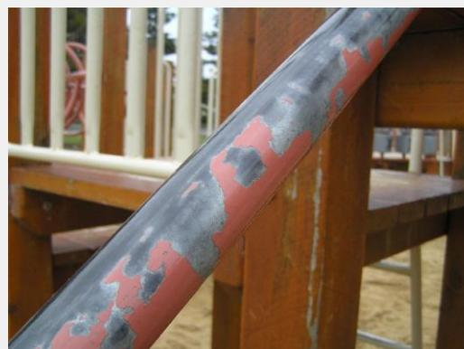
*The smooth surface provided no key for the coating system to adhere to*
