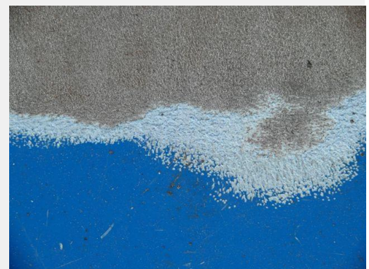
The MBX ® Bristle Blaster ® creates a measurable profile
