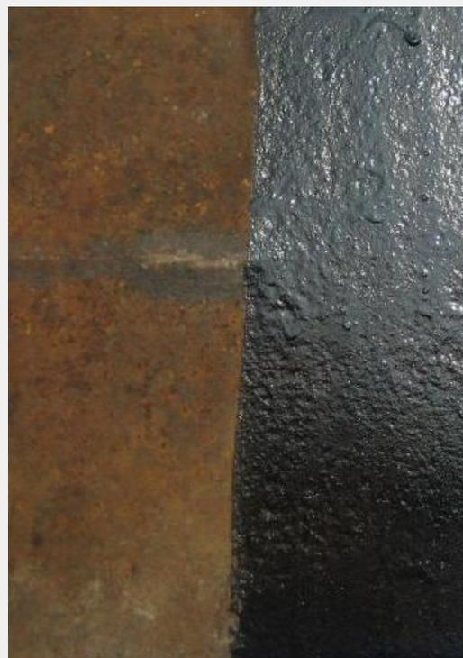
*Rust converters are not recommended for structural steel according to AS2312*
