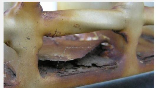
*Millscale is a common cause of premature rust and must be removed prior to painting*
