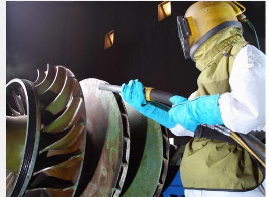
*Abrasive blast cleaning is the most effective and fast way of removing millscale and other contaminants*
