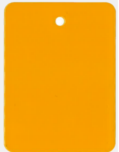
Colour samples in the specified product and signed off by the project manager avoids disputes about expected colour later. Fan decks should not be relied upon for colour checks.
