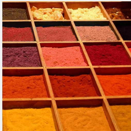
Colour is delivered by either grinding the coloured pigment into the base paint at manufacturing stage or by adding tinter to the product at point of sale.
